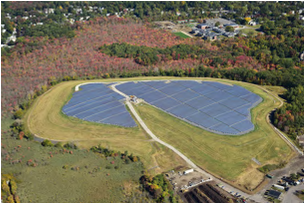
Figure 7.5 Credit Brightfields Development, LLC. Neeham, MA 13-acre landfill converted into a brightfield. It provides 30% of the town's energy. Source: http://solarbrownfields.com
